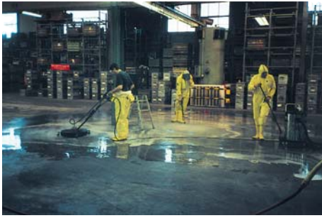
First Cleaning process, VAP 1® ORS-D Detergent.
